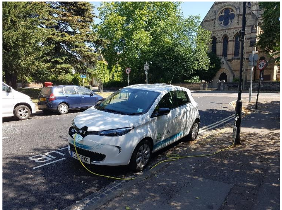
A car-club vehicle charging from a converted lamppost in central Oxford.
