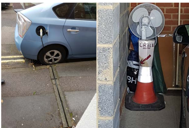
Figure 2. Two examples of how trial participants used temporary and informal measures such as road cones and rain drains to reduce the chances of someone tripping on the cable while charging their electric vehicle. Picture taken by: B. J. Doody.
