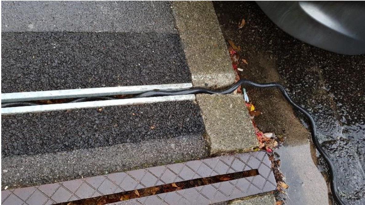
Figure 7. A few of the participants using the home charger reported that the allocated cable began to show signs of deformation reasonably early into the trial. The extent to which different users cables have become twisted and deformed has varied as the trial has proceeded. William has suggested that it has become harder to feed his cable pictured above into the channel as it has become more twisted. Picture taken by: Trial participant William.
