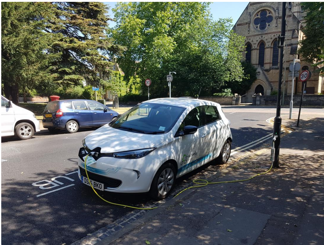
Figure 13. A Co-wheels' Renault Zoe charging using an Ubitricity lamppost charger. Users noted that the cables might make the cars more vulnerable to vandalism and create a potential trip hazard.
