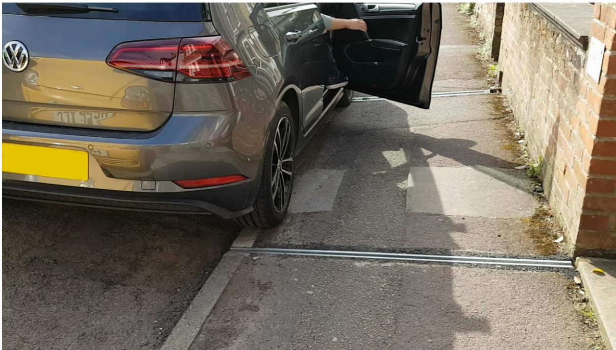
Figure 5. A video still highlighting how, whenever possible, Oliver parks his car so that the rear of the vehicle is positioned over the top of the cable channel. He suggests that this helps to further reduce the trip hazard associated with the cable. Video recorded by: B. J. Doody.
