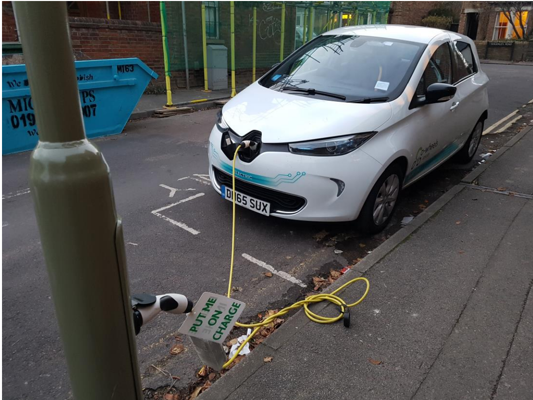
Figure 12. A Co-wheel's Car Club Renault Zoe charging using an Ubitricity lamppost charger. Users noted that although it is a relatively simple process, the cable can be somewhat cumbersome, bulky and unpleasant to use and store.
